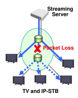
Packet loss can not be allowed in commercial contents delivery
