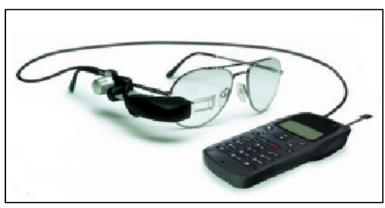
MicroOptical Clip-on Display VGA resolution Color
