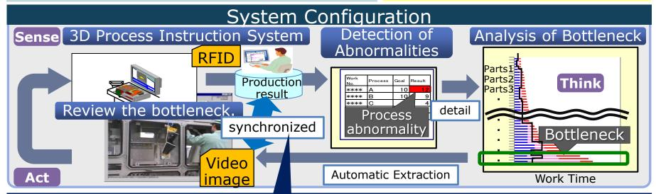
The Video Analyzing system is synchronized with Work Process Data linked by RFID.
