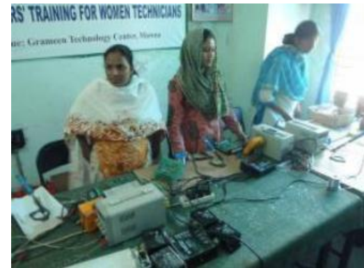
Female Workers Producing SHS Control Panels
