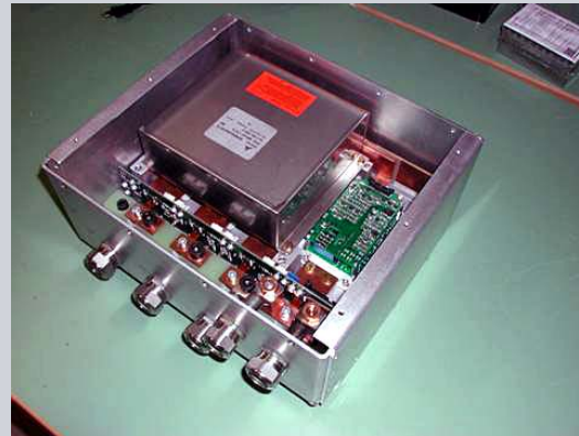
integrated inverter & charger
